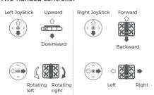
The illustration displays the two-handed controller in the default operation mode (model 2). You can change the controller mode in the system settings.
