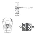
Press and hold the Motion Button to activate gesture control.
