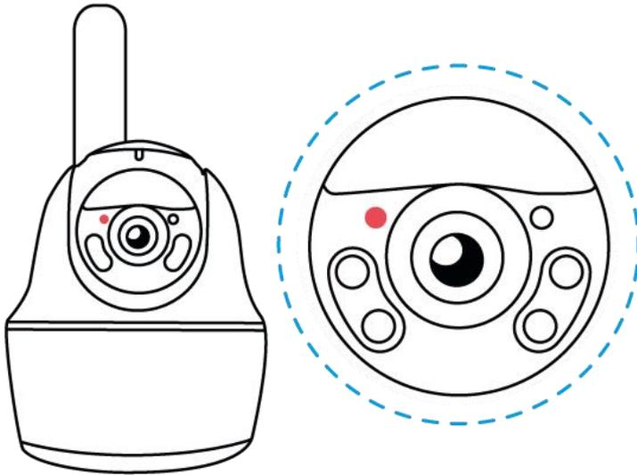
3. A blue LED will flash for a few seconds and then go solid before going out. You will hear a voice prompt "Network connection succeeded", which means the camera has been successfully connected to the network.
