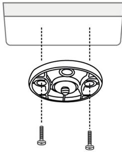
**Step 2.** Align the camera with the bracket and turn the camera unit clockwise to lock it in position.
