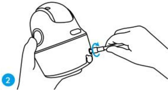
**Note:** In order to get a better network connection, it is recommended to install the antenna upward or horizontally.
