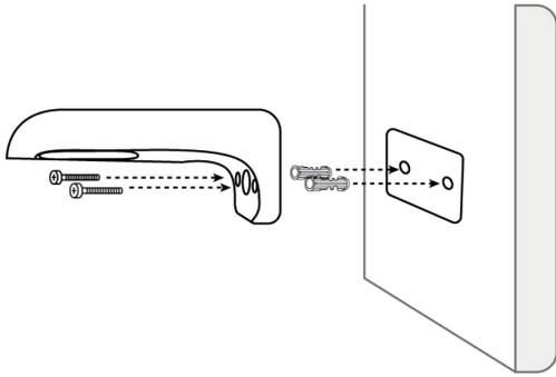
**Note:** Use the drywall anchors included in the package if needed.
